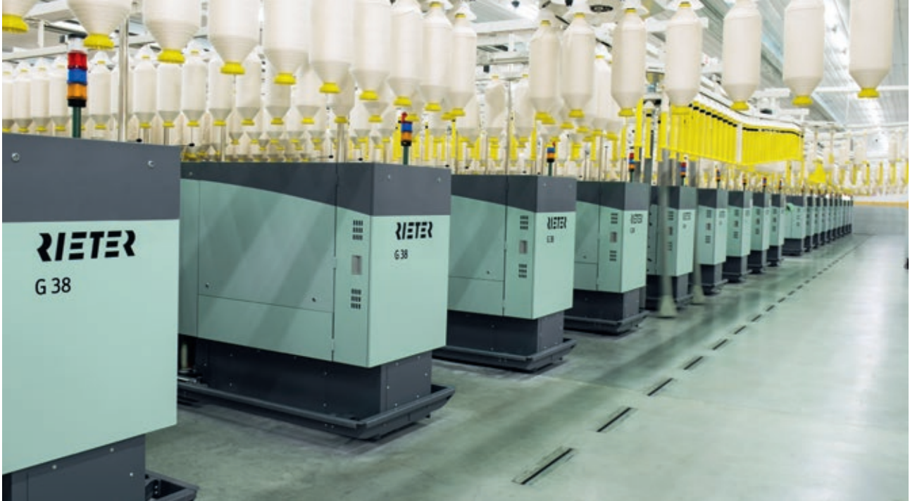
The G 38 ring spinning machine is one of four new spinning machines. It offers a maximum degree of automation as well as best yarn quality coupled with maximum productivity and complete flexibility.
