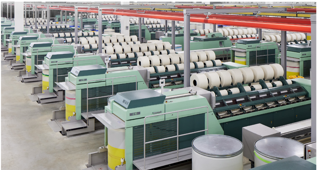
The new machine layout allows a 11% closer machine placement
