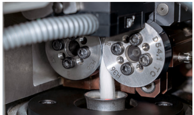
Sliver jam is straightened by turning the coiler to avoid sliver jam at restart
