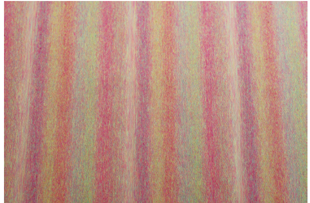
Fig. 4a: Sample using fancyflex VARIO 3 colors with long-changing times
