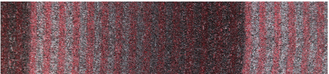
Fig. 5b: Sample using fancyflex VARIO 3 colors without intermingling option
